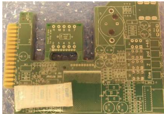
Gold Finger, Through-hole FR4 PCB Vacuum Packaging with Desiccant
